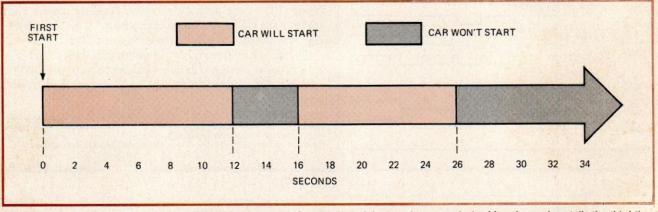
2. Timing. The start-stop cycles for the anti-theft device are 12 seconds and 4 seconds, respectively. After the engine stalls the third time, it can not be restarted until the driver opens the enable switch S<sub>1</sub>, which is concealed within the car's interior.
